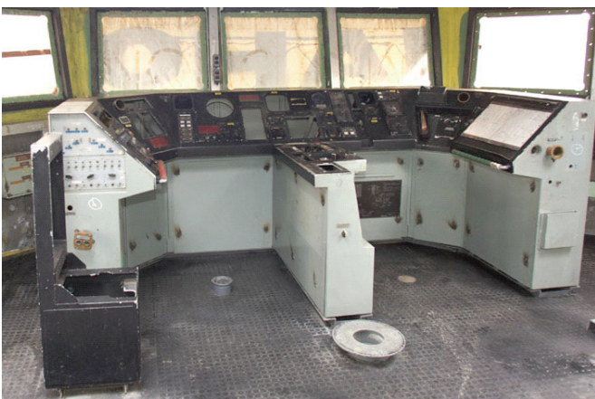
Figure 2: Bridge console and instrument panel
